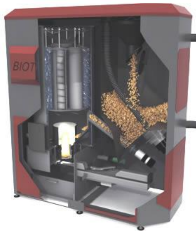
Fig. 7: Wood pellet boiler.
