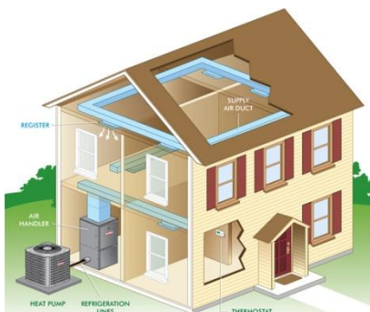
Fig. 6: Ambient air/water heat pump system.
